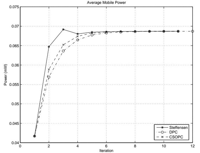
Fig. 2. Performance comparison of average powers calculated using DPC, accelerated DPC, and CSOPC in a CDMA cell with 10 users with  $\gamma_i^{tar} = 5.0$  (7 dB) for all mobiles
