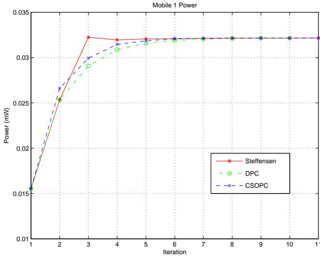
Fig. 4. Performance comparison of powers calculated using DPC, accelerated DPC, and CSOPC for a typical mobile (mobile 1) in a CDMA cell with 10 users with  $\gamma_i^{tar} = 5.0$  (7 dB) for all mobiles
