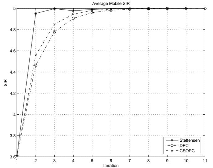
Fig. 3. Performance comparison of resulting average SIRs for DPC, accelerated DPC, and CSOPC in a CDMA cell with 10 users with  $\gamma_i^{tar} = 5.0$  (7 dB) for all mobiles
