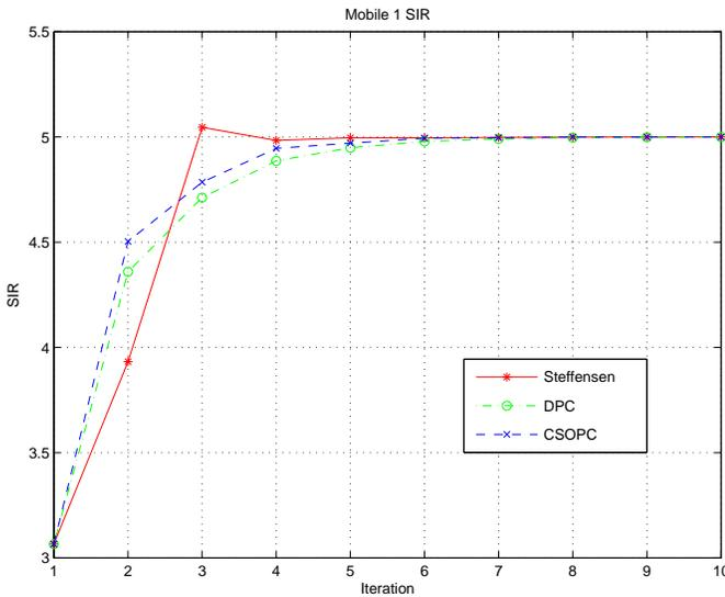
Fig. 5. Performance comparison of resulting SIRs for DPC, accelerated DPC, and CSOPC for a typical mobile (mobile 1) in a CDMA cell with 10 users with  $\gamma_i^{tar} = 5.0$  (7 dB) for all mobiles
