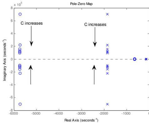
Fig. 7. Root-locus for variation in Capacitance
