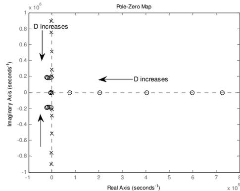
Fig. 6. Root-locus for variation in duty cycle
