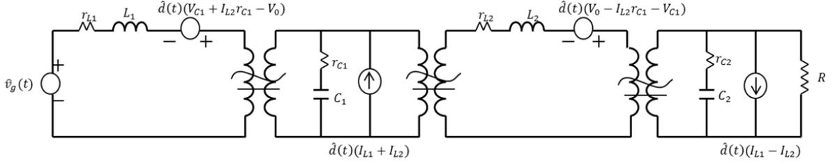
Fig. 3. Schematic diagram of Small Signal Model of the SEPIC Inverter when operating to produce negative cycle of output
