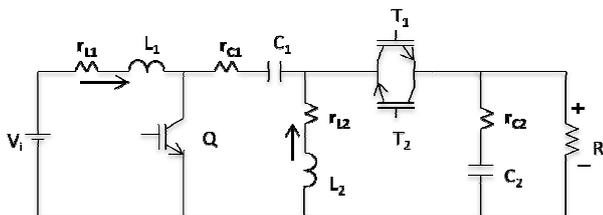
Fig. 1. Schematic Diagram of the New SEPIC Inverter
