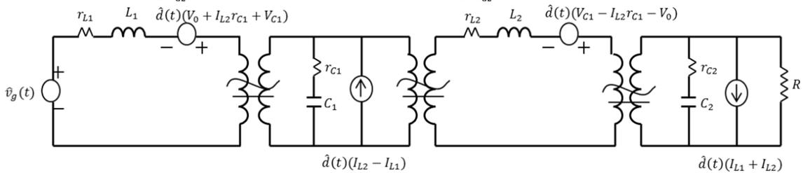
Fig. 2. Schematic diagram of Small Signal Model of the SEPIC Inverter when operating to produce positive cycle of output
