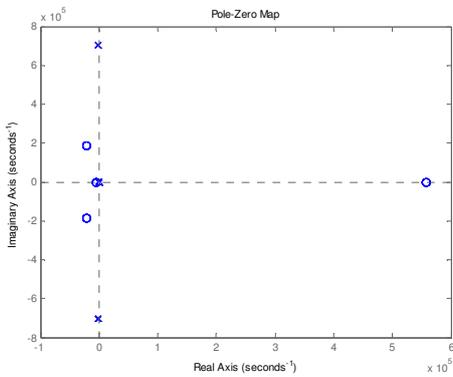
Fig. 4. Root-locus for variation in Capacitance
