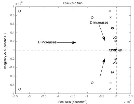
Fig. 9. Root-locus for variation in duty cycle
