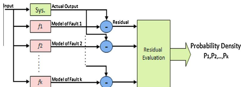
Fig. 4. Multiple-model residual generation and residual evaluation.
