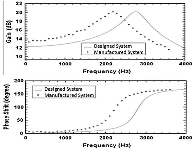
Fig. 3. The frequency response (Bode-plot) of the simulated designed system and the measured values from a fabricated MEMS LCR [17].
