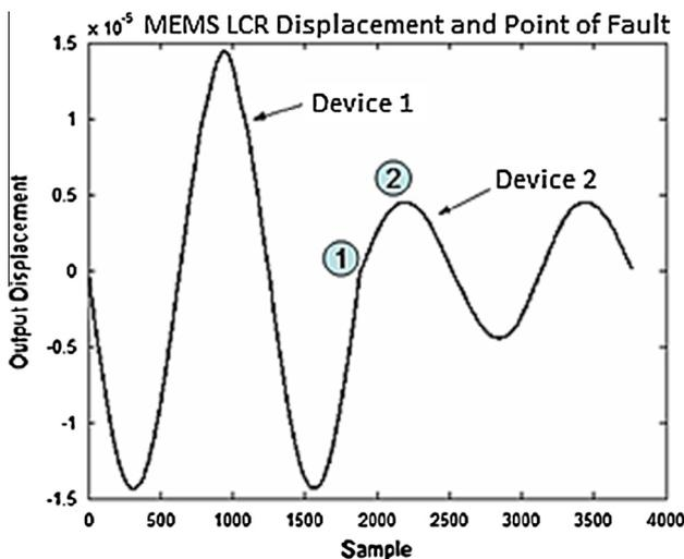
Fig. 5. Displacement of LCR and the point of fault. Point 1 determines the location of the fault, and point 2 determines the first peak of the second system output.
