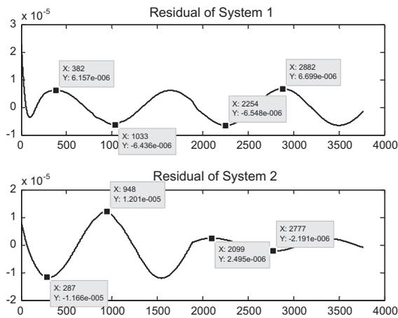
**Fig. 7.** Residual signals generated for device 1 and device 2. A lower residual signal from samples 0 to 1886 was obtained from device 1 and from samples 1886 to the end from device 2. The maximum and minimum of each residual section is shown in the figure.
