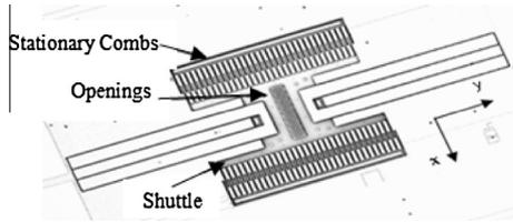
Fig. 1. MEMS lateral comb resonator.
