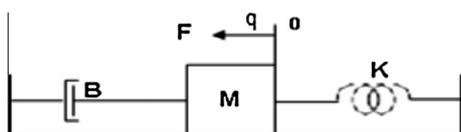
Fig. 2. Mass-spring-damper, schematic model of lateral comb resonator.
