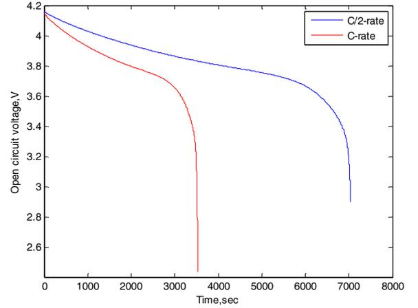
Fig.3. Open circuit voltage of Li-ion battery
