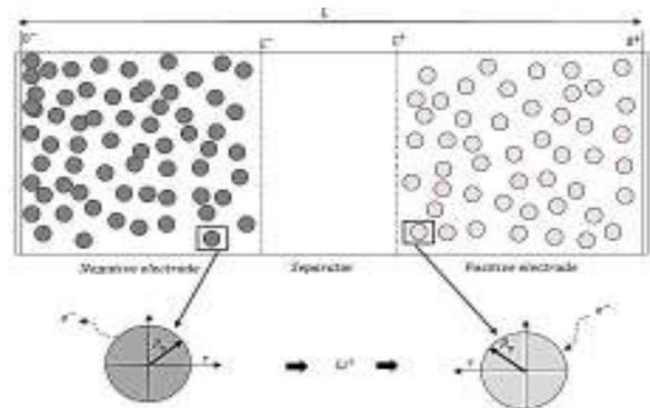
Fig. 1: Schematic Li-ion battery geometry [1].
