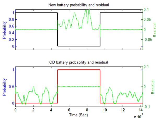
Fig. 8. Conditional probability density and residuals evaluated for new and OD battery condition
