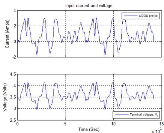
Fig. 6. UDDS load/charge current and terminal voltage profile
