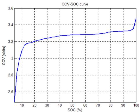
Fig. 2. OCV-SOC curve for LiFePO<sub>4</sub>
