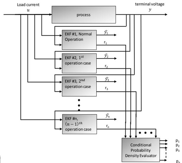
Fig. 3. Multiple-model residual generation and probability evaluation
