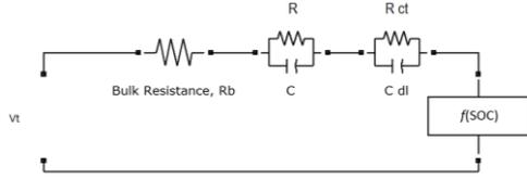
Fig. 1. Li-ion battery equivalent circuit model
